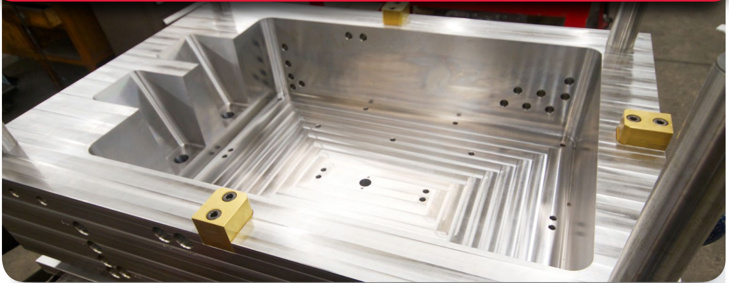
We engineer hybrid tooling to combine shorter cycle times with tool durability (which means no increase in preventive maintenance requirements compared to P20 tools).
