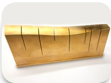
A fixed insert for the core side of a thermo-plastic injection mold, made with MoldMax to ensure localized cooling for deep ribs.
